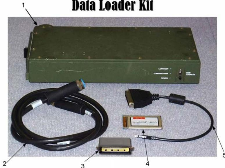
The parts required to connect the SDTMR are: (1) Transfer Unit (2) Cable Assembly, Power (3) Dummy Load Terminator (4) Cable Assembly, SCSI PCMCIA Card (5) SCSI PCMCIA Card
